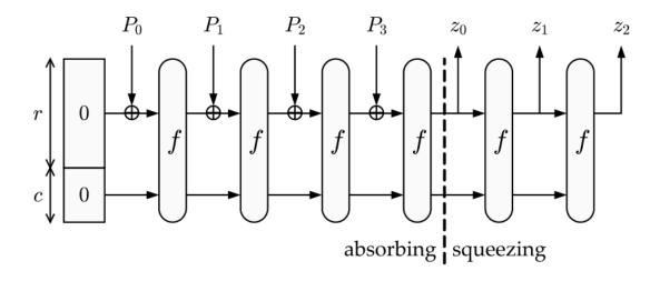
Note that for CictroHash the digest will simply be the value  $z_0$ . Also, for CictroHash r is 4 bytes in length and c is four bytes in length. The starting state of r and c (denoted S) is shown below.
